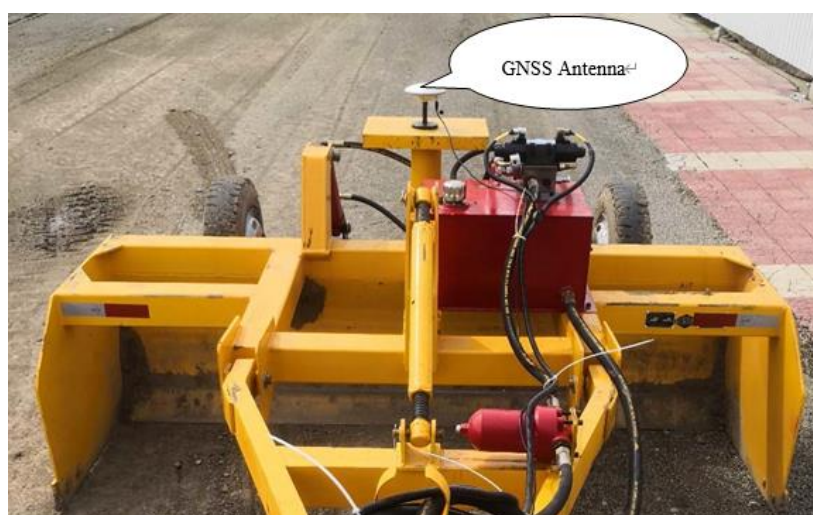
Figure 2.1 GNSS antenna installation
